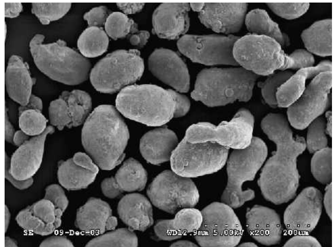
Fig. 5 Morphologies of the gas atomized aluminum powder particles
